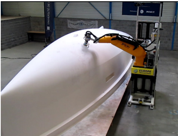
Autonomous moving platform, mould sanding automatic process
